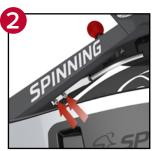
STEP 2: Using a 4mm allen wrench, carefully remove the two bolts supporting the brake pad (indicated with red arrows). Remove the old brake pad assembly.
