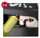
**STEP 5:** Turn the resistance knob clockwise until the flywheel is locked and cannot rotate. With the flywheel locked, spray the lube onto the chain. Loosen the brake and rotate the crank carefully and slowly, by hand, approximately an eighth of a turn, and then lock the flywheel again. Spray lube onto the next portion of the chain. Repeat the above steps a total of eight times to lubricate the entire chain.
