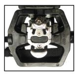
The SPD pedals are set for the lowest release tension at the factory for safety. If you would like a stronger release tension, use a 3mm allen wrench and turn the adjustment screw clockwise. Adjust both the left and right sides evenly and start with as little adjustment as necessary until you achieve the desired release tension.
