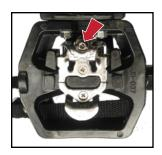
The SPD®-compatible pedals are set for the lowest release tension at the factory for safety. If you would like a stronger release tension, use a 3mm Allen wrench and turn the adjustment screw clockwise. Adjust both sides evenly and start with as little adjustment as necessary until you achieve the desired release tension.
