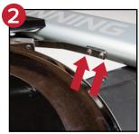
**STEP 2:** Using a box wrench, carefully remove the two bolts supporting the brake pad (see red arrows left). Remove the old brake pad assembly.
